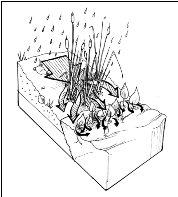
Fig. 9-4. Schematic showing how wetland plants intercept and slow down flowing water during storms.
